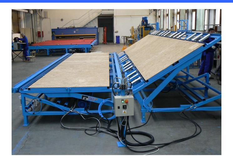
Turning Table is a highly satisfactory and cost effective way of producing sub components, walls, or complete houses for that matter. The table comes in the following lengths: 12 m, 10m and 8 m. Wall height can be adjusted from 2200 mm to 3800 mm and is pneumatically aligned to ensure each wall is assembled straight.
