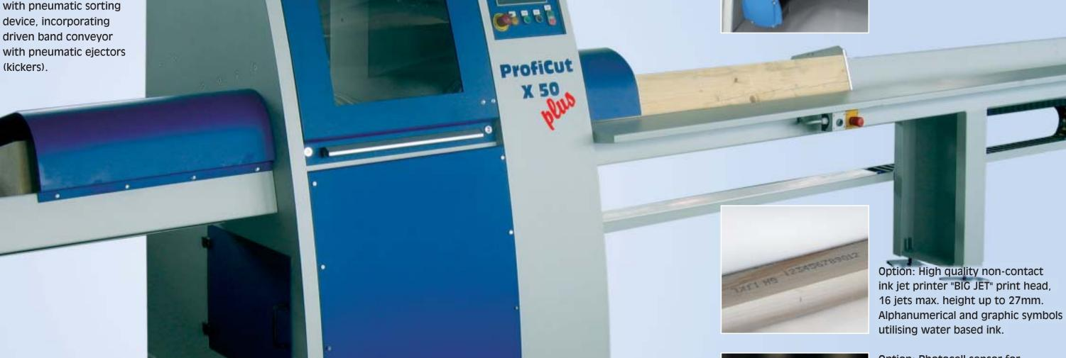
Option: Photocell sensor for automatic length recognition with full optimising software for maximum length, priority length, minimum waste and volume. Photocell sensor for use with fluorescent crayon for detecting and removing defective parts.
