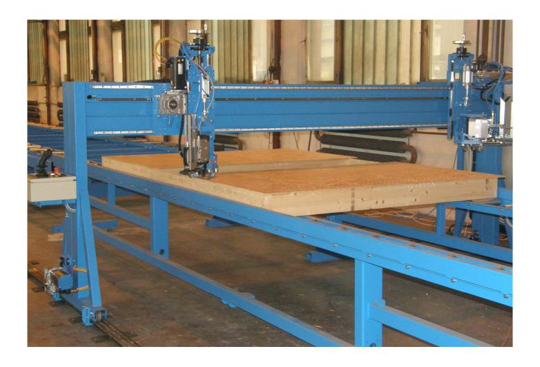
The Sheeting Bridge takes on the job of fastening with only two tools, but what smart tools they are. With operate panel and easy software "self teach mode" simplicity and functionality are combined to deliver maximum flexibility, maximum up-time and maximum results, all with the touch of a button. Movable wagon with tool is power by servomotor and position on the wall frame is very fast and exactly. Together Sheeting Table is ideal assembly for produce of wall panel.
