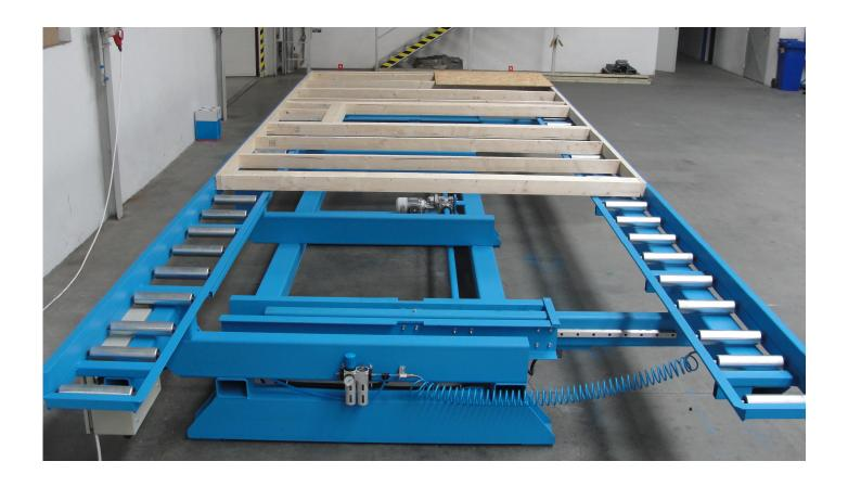
The Sheeting Table is the foundation of Sheeting Bridge. It acts as a working height platform, product squaring device and material-handling conveyor. The Sheeting table features powered width adjustment for rapid changes to diffirent wall heights and swing gates that allow for greater single operator access through the machine.
